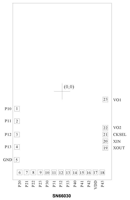
Note: The substrate MUST be connected to Vss in PCB layout.
